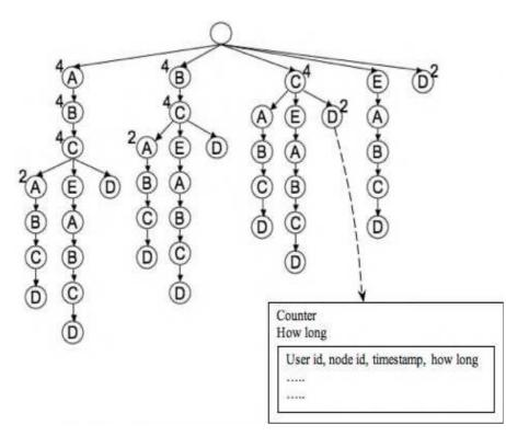
**Fig.1** - Suffix tree containing two trails, namely ABCABCD and ABCEABCD.Each letter represents a wireless sensor nodes with which at least one robot has interacted with. Each node is also associated with additional metadata used to answer and rank significant trail queries.
