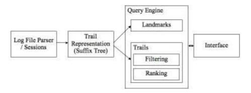
**Fig 2** – Coordination engine architecture. From left to right, a log file is parsed for correctness and in order to ensure that there are no violating transactions. Then the parsed interaction logs are transformed to our representation – namely the Suffix Tree. The next step is the filtering and ranking of the trails. On the far right, the User Interface can be used to submit arbitrary queries that will in turn consult the data structure to formulate the results.
