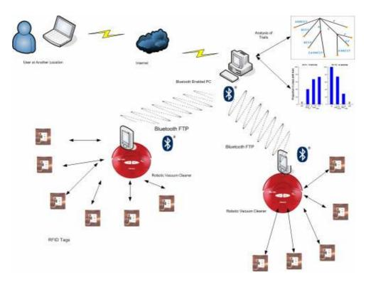
**Fig. 3** – High-level depiction of a version of our system. The round objects represent the robotic cleaner which is augmented with the surrogate device that reads and logs interactions with the RFID sensors (square objects in the figure). Information is transferred wirelessly via Bluetooth (although other alternatives may be used e.g. Wi-Fi, Zigbee, etc) to a desktop-class PC or a mini server. The PC or mini-server continuously processes and filters the information,
