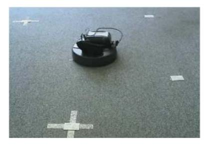
**Fig. 4** – iRobot Roomba Robotic Cleaner with Surrogate Device mounted on top of it. Also visible in the picture, are the RFID tags attached to the floor, forming a proximity grid.
